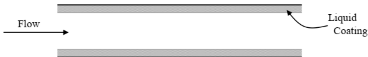
Figure 2. Liquid phase coated onto the inside walls of a capillary column
